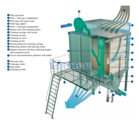
For cleaning vent of flue gas emissions and remove particulate matter & control of SPM level Unit has been designed & manufactured as per joint prior discussions & technical concurrence on parameters like Air to cloth ratio, Can velocity, Dust loading, Existing & new bag cage sizes, Heaters, Control system, Inlets/ outlets etc.
